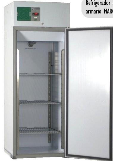
0/+8°C, one solid door, ANTIBACTERIAL STEEL INTERIOR, FORCED cooling and AUTOMATIC defrost, grid shelves included, door lock, microprocessor controller with temperature and door open alarms, contact for remote alarm
